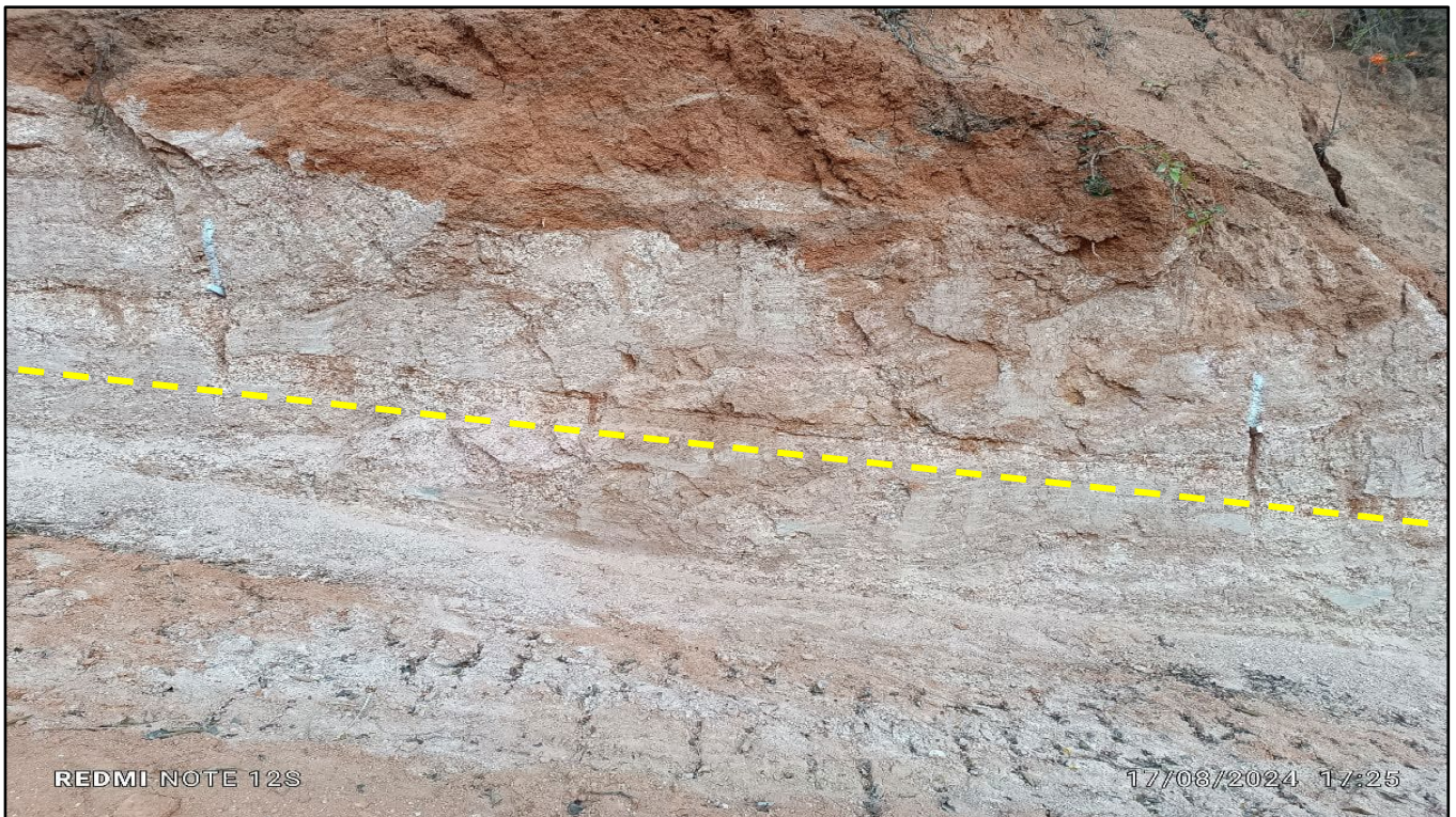
Figure 3 – Channel sample CLD-CHN-006 taken from road cut at entrance of artisanal workings, returned 5,460ppm TREO from 15 to 20 meters width
