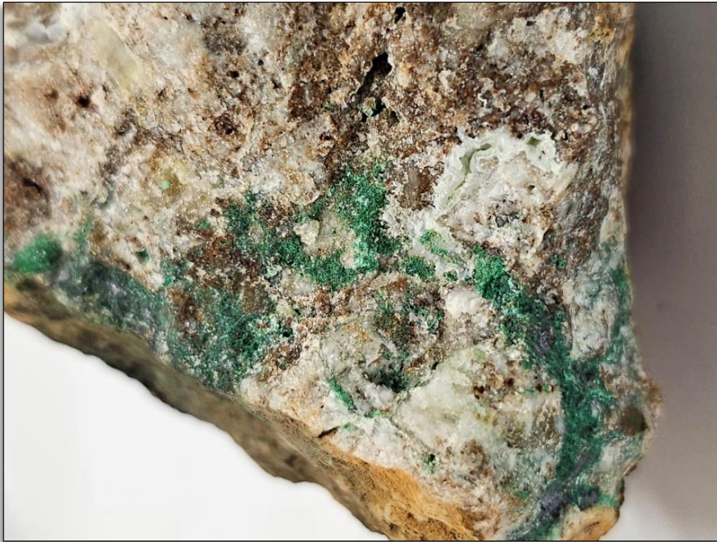
Figure 2: Sample AR28581, Piper prospect quartz breccia. Assays of 9.5% Cu and 1.7g/t Ag. Field of view; 5cm.
