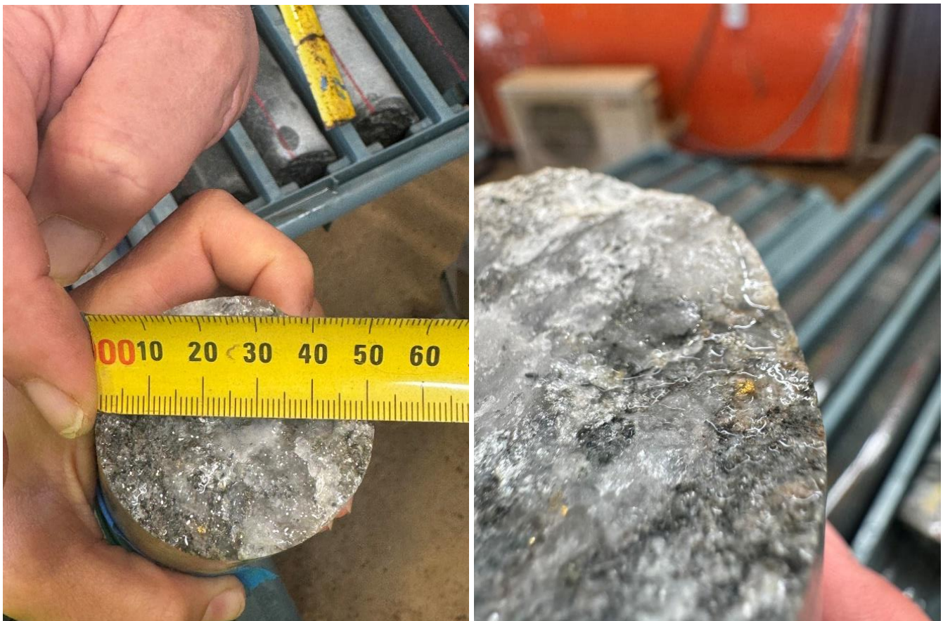
Figure 3: Free gold on minor veining in Lady Herial DD hole FOS24DD_012 5 – the interval assayed 20.54g/t Au over 0.35m.
