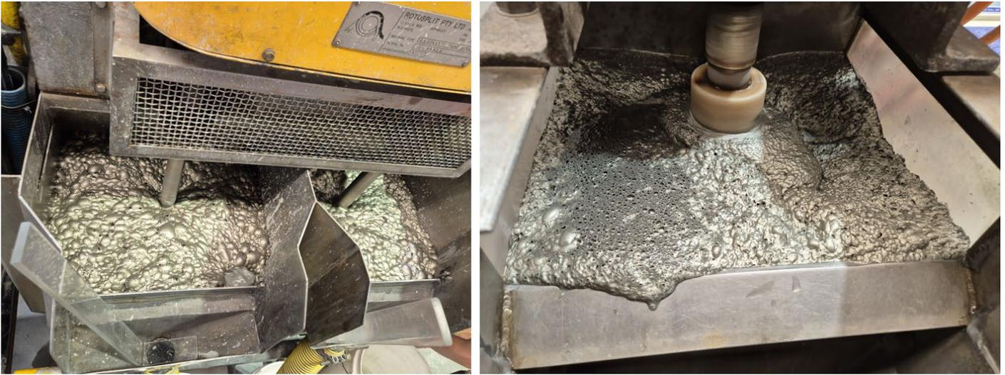
Figure 6: Metallurgical composite rougher flotation (left) and cleaner flotation (right).
